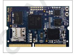
The BAV335x is provided as a small board to be used with a single low profile, SODIMM mating connector. The module makes it easy for OEMs to integrate Texas-Instruments' powerful Sitara processor in their designs without having to worry about complex EMI and PCB layout typical of BGAs fine pitch designs, high-speed DDR3 with impedance and trace length matching considerations.
